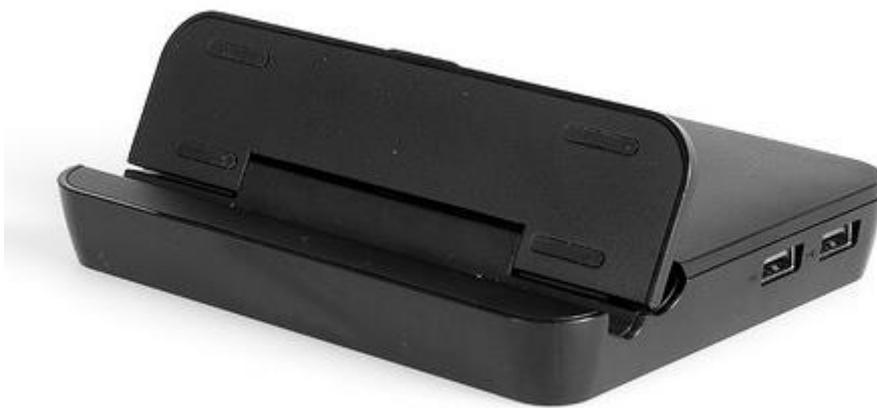
This is a small but full-featured docking station that provides the BMxPad with four USB 2.0 ports, one LAN 10/100 port and one HDMI port. A nice solution that transforms the tablet into a true desktop computer once it's connected to its docking station. A keyboard and mouse can be attached to the docking station, as can a printer, scanner, and of course a larger monitor.
