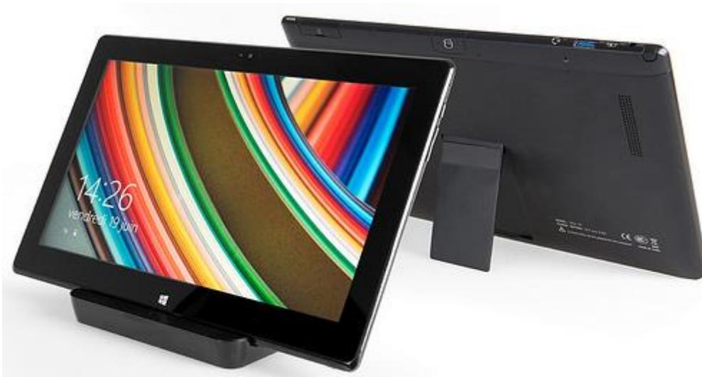
The device is powered by a range of Intel processors up to and including the Intel Core M-5Y10c. It can hold up to 8 GB of RAM and 512 GB of SSD storage. It has 802.11AC wireless connectivity, supports Bluetooth 4.0 and can take on a 3G or 4G modem.
