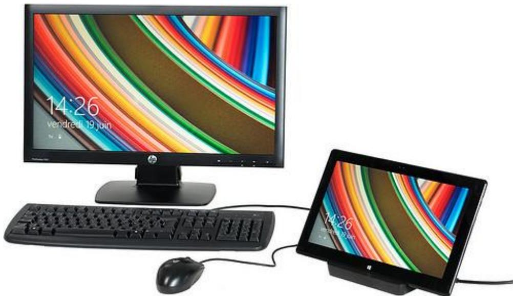
The tablet itself has a wealth of connections, with a few features that are currently not available at all on the major brand models: one full-size USB 3.0 port, one MicroSD card slot and one MicroHDMI 1.4 port, which can take on many external devices. An active stylus with pressure response management, which can be stored in the tablet, is also available. And finally, a stand housed in a semi-reinforced shell allows you to position the device vertically, without needing the docking station.
